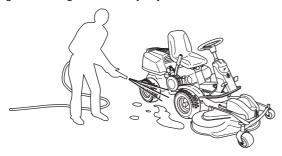
Oily dirt can be removed using a cold degreasing agent. Spray on a thin layer.
